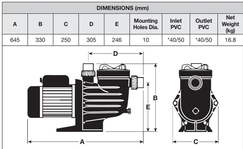
\* Suction & delivery accept both 40mm and 50mm PVC pipe.
